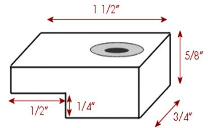
The stand should have a 5/8" hole drilled in it for the brass fitting on the vacuum controller. Then connect a piece of tube from the fitting on the main reservoir to the vacuum controller (through the hole). The image on the right shows a piece of black tubing from the vacuum controller to the main reservoir.
