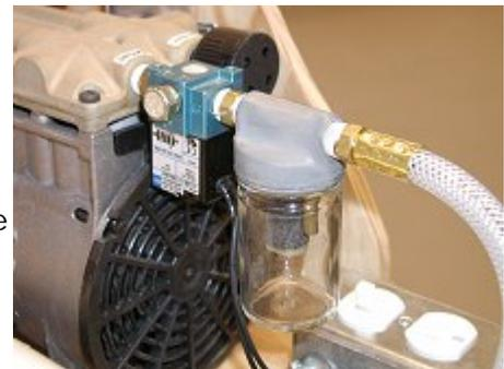
**Please note:** Be sure to use the vacuum or "intake" side of the pump. Using the output side will immediately ruin the diaphragm inside the vacuum controller when the system is first turned on.
